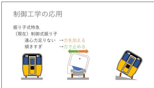
Fig.15 Explanation of body tilting device (2) (Step.4)
